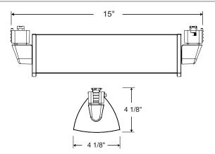
Alternate HTYPE Trac Adapter Compatible with track systems which use a H-type track adapter, including Lithonia LTS Decorative Track (not LT type) • System specific and assembled to trac fixture • Two-position power contact provided for two-circuit application • Consult factory for additional information.
