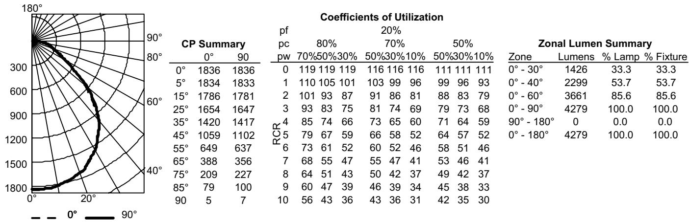
2GTL4R 48L EZ1 LP835, 5027 delivered lumens, test no. LTL3102P4, tested in accordance to IESNA LM-79
