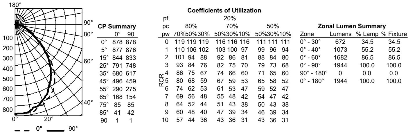
2GTL4R 40L EZ1 LP835, 4278 delivered lumens, test no. LTL3102P0, tested in accordance to IESNA LM-79
