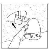
Step 2: Using provided wire connectors, connect wires (black to black; white to white; ground to ground) and insert housing into ceiling.
