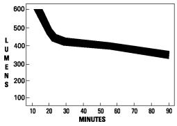
Light output data based on two F40 CW lamps (3050 lamp lumen rating). Two-lamp energy-saving rapid start ballast. Thermal and ballast factor corrections have been included. Light output for other lamp and ballast types will vary. Luminaire efficiency and application conditions must be determined to calculate actual illuminance levels. Consult Lithonia Lighting represenative for further information.
