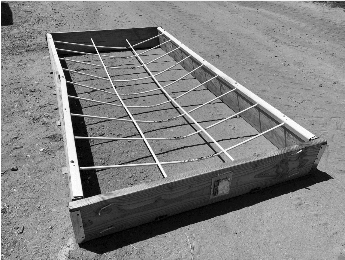
Photo No. 1 After impact load testing, 400 lbm dropped 42"
