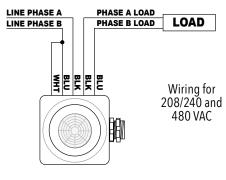
**Note:** Once installed, the sensor may take a few minutes to become active. Additionally, there is a 45 second delay before switching from off to on (this delay is 55 seconds when connected to 50 Hz).
